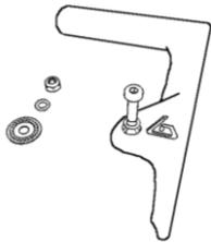
1.d – Put one O'ring on the 20mm screw, slot them both into the hole provided in the stock.
